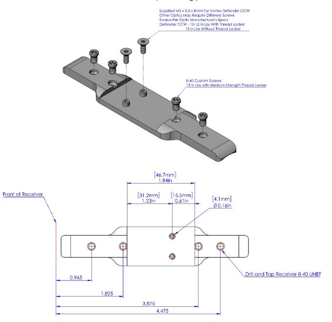
This hole spacing is consistent with factory Benelli M4 and M2 Tactical hole location. This distance from the front of the receiver is the preferred location for the optic mount, however any position on the receiver will work if the hole spacing is correct.
