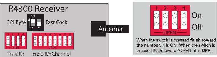
Each individual switch is labeled with a number. These numbers ARE NOT VALUES. **Switch 1 has a value of 1, switch 2 has a value of 2, switch 3 has a value of 4, and switch 4 has a value of 8**. Add the VALUES of each switch in the ON position to get the Trap ID. Below is a chart with the switch values and examples of the different dip switch sequences.
