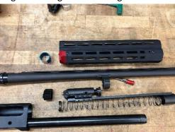
Install the supplied blue ring onto the magazine tube, with the flat silver face on the top towards the bolt carrier, and reinstall the recoil spring, bolt carrier, and bolt per the owner's manual.
