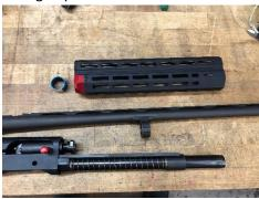
Remove the bolt, carrier, recoil spring, and the black plastic handguard alignment ring from the magazine tube.
